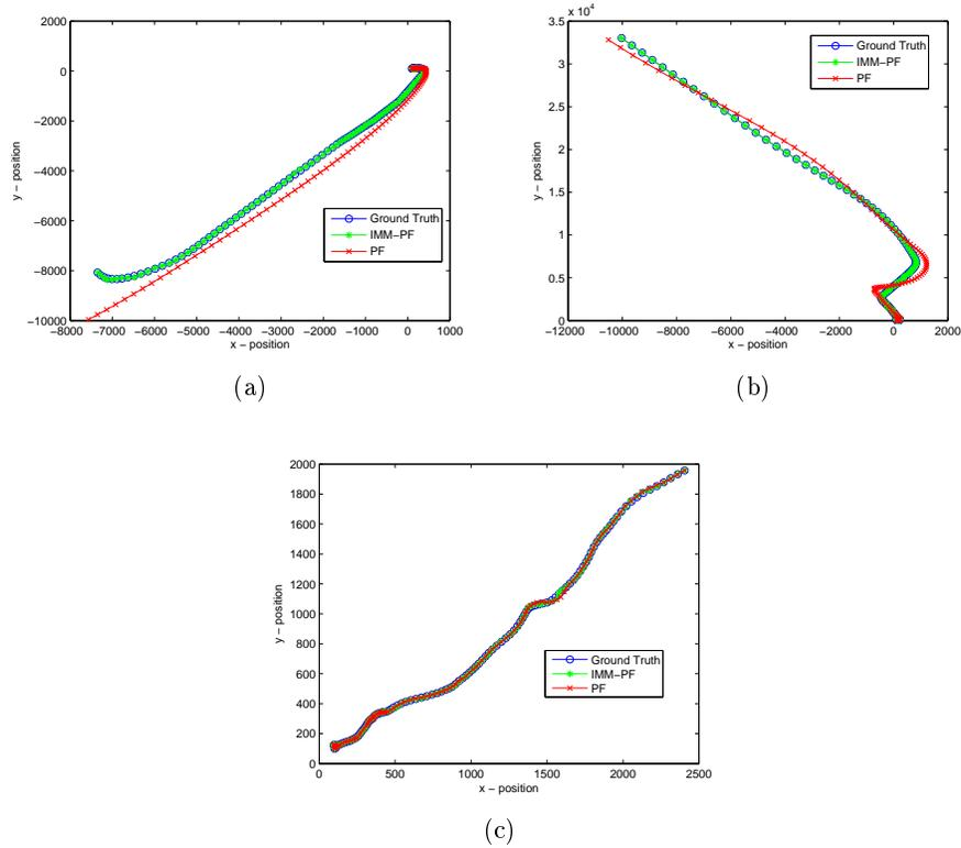
Fig. 1: IMM – PF compared to PF : Fig. (a) Simulation with  $\sigma_{vel}^2 = 1$ ; Fig. (b) Simulation with  $\sigma_{vel}^2 = 10$ ; Fig. (c) Simulation with  $\sigma_{vel}^2 = 100$ .
